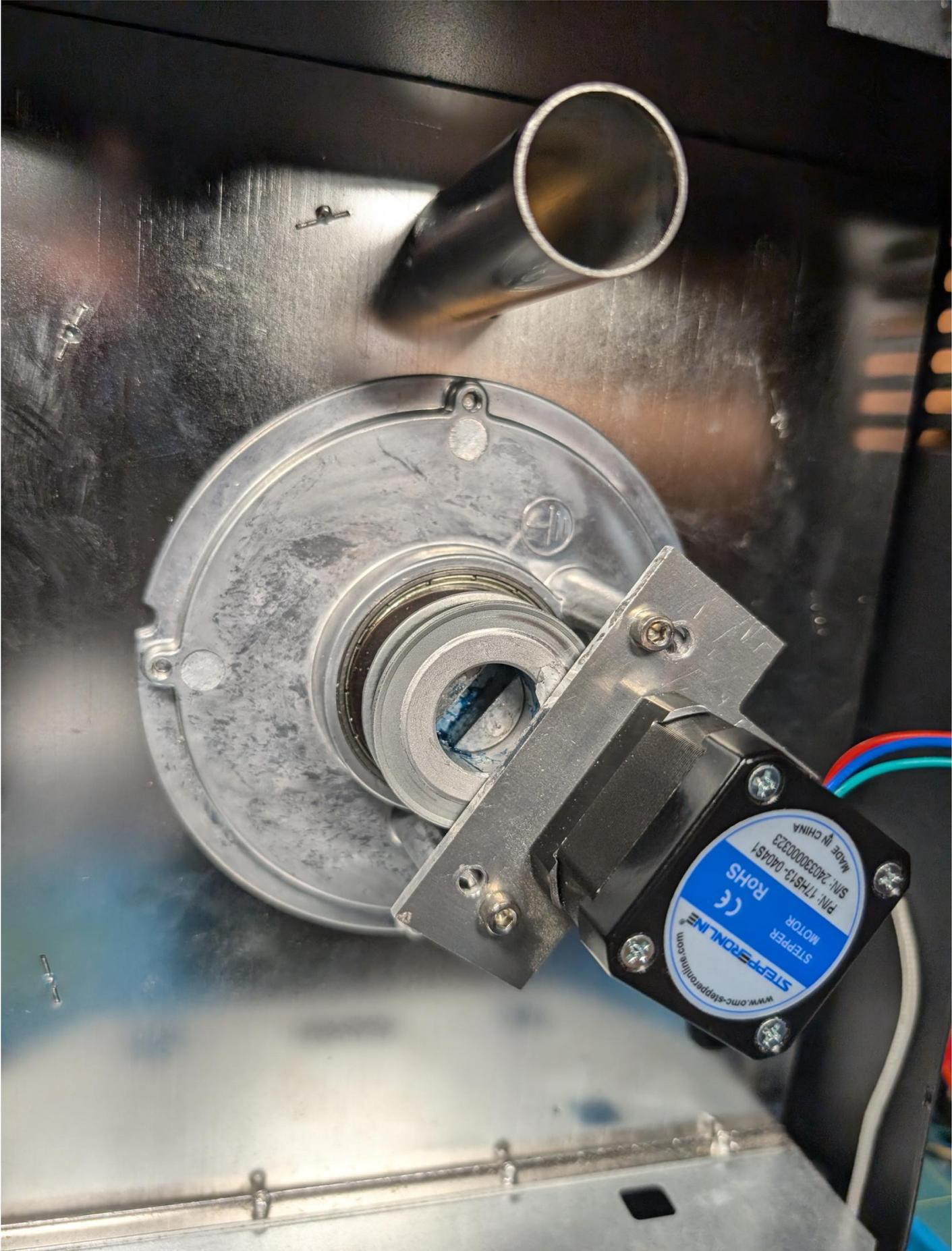
Fits with modified electronics box. Quieter than stock RPM controllable via Artisan.
