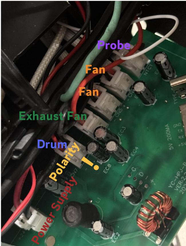
**POLARITY WARNING! Double check Polarity on Drum connection as the wire color is not depicted accurately of VCC and Ground (In picture the red wire is on ground(-) and the black wire is VCC(+))**
